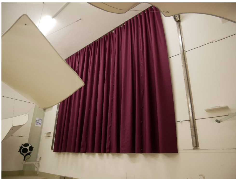
Figure B.2. Test object in the reverberation room: Pleated arrangement, diagonal view.
